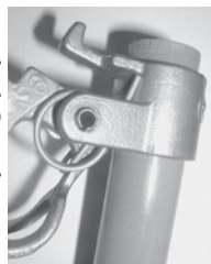
MECHANICAL ASSIST: FUSEHOLDER IS AVAILABLE WITH A TORSIONAL SPRING ON TRUNNION TO AID DROP OUT OPERATION IN CORROSIVE ENVIRONMENTS.
